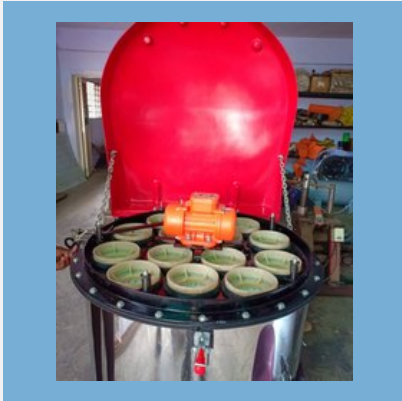
Cement Silo Top Mounted Dust Collector
