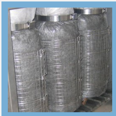
Dewatering Sludge Bag
